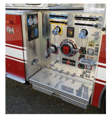
New aluminum slide out step under the pump panel to reduce corrosion.
