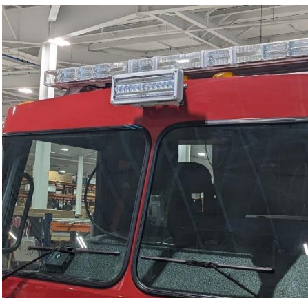
Figure 3 & 4: New FRC Spectra Brow Light Bracket (will not have Sutphen logo cutout)
