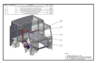
Example Diagram of New Cab Coolant Lines
