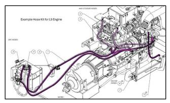
Example Diagram of New Engine Hose Kit
