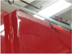
In addition to the top edge of the wet side tank, the area behind the side mounted porta tank racks on the wet side tank will be finished with color coated raptor.
