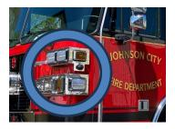
If a customer chooses Option 2, Sutphen will remove the camera bracket from the top headlight housing and mount the camera directly to the side of the lower headlight housing. You can see this specification in the images below:
