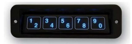
The manufacturer Essex Electronics has informed us that they will be discontinuing the option for red backlighting for the keyless entry touch pads. From this point forward the only option will be the blue backlighting seen above.
