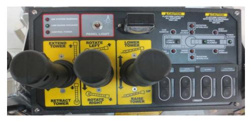
Using the JC1500-034 joystick (Operator Presence) also requires a different Base and Basket controller with more inputs as a result of the operator presence wires. The new Base and Basket controller are a little larger but we are able to mount them in the same locations without any issues.
