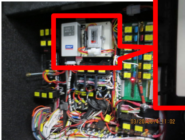
Example of Electrical Panel on Heavily Optioned Apparatus Requiring Options to be Stacked on Top of Each Other
