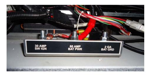
An additional set of three (3) power & ground studs will be offered as an option in the lower command console. This option will also include one (1) 60A battery power, one (1) 30A ignition power, and one (1) 125A ground. You will see this option become available with the next release of data to the configurator/SQS2.
