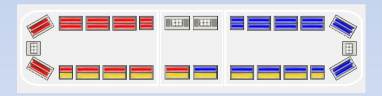
55" models: 8 long and 2 short Inboard Linear-LED® modules
