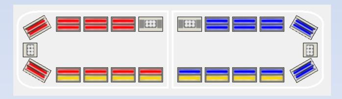
49" models: 8 long Inboard Linear-LED modules
