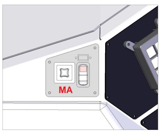
Position #MA will be remote mirror adjustment knob and mirror heat switch (if selected).
