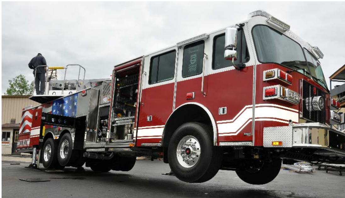
1.5 x Rated Load Overturning Test
