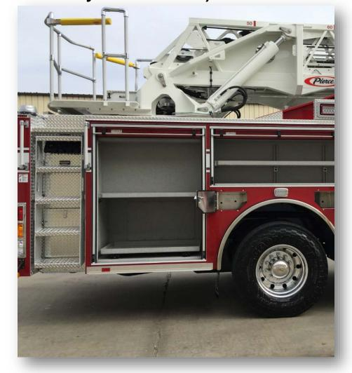
Fold-out step assembly – Was rather difficult to pull out and is very sensitive to be stowed perfectly or triggers sensor in cab.
