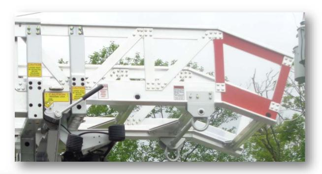
The ladder will be designed to provide continuous egress for firefighters and civilians from an elevated position to the ground. The end of the fly section will be constructed in a manner that aids personnel in climbing off the ladder.
