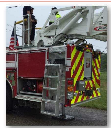
The turntable is accessed from the side of the truck (driver's side only or both sides).
