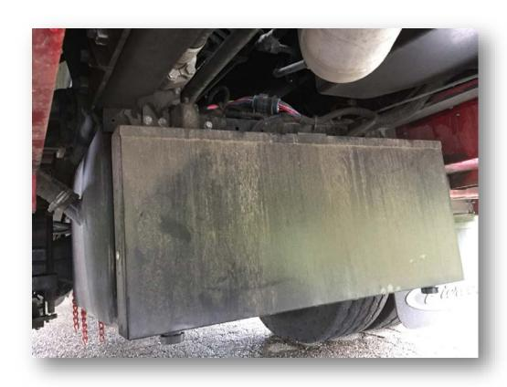
Electrical distribution box is underneath the apparatus behind the fuel tank.
