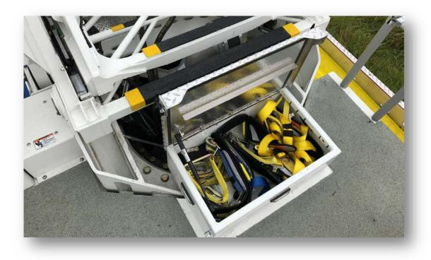
The turntable is pretty large and the first step incorporates a storage compartment for ladder belts, etc.
