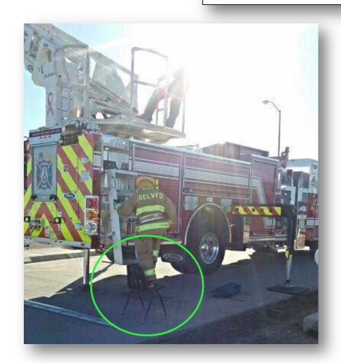
If the unit is set up on an incline, step height can become compromised. That bottom step looks much higher than 24".
