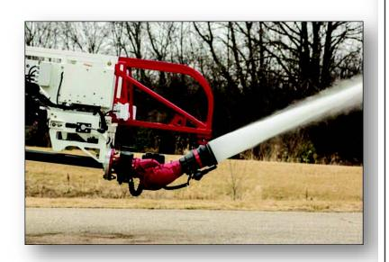
**ZERO** tip load capacity when flowing nozzle above horizontal.
