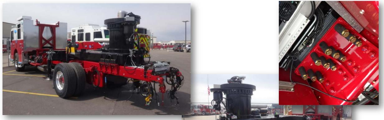
Torque box is mounted to the chassis frame rails in 4 locations (one each side under outriggers and one each side behind rear axle.
