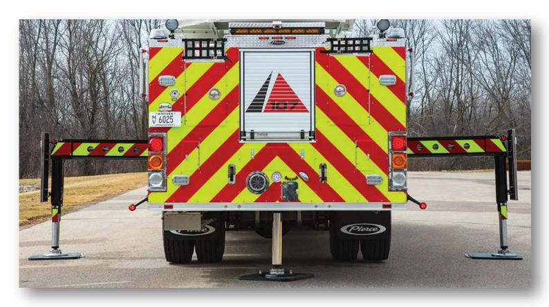
**Fully Deployed Outrigger Spread = 18'**
