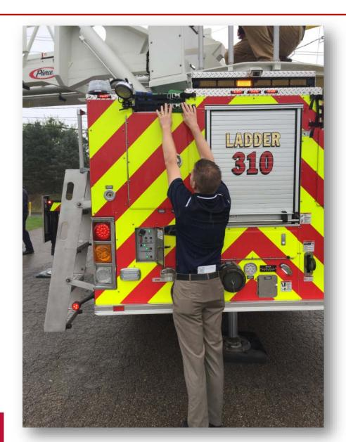
With the truck up on its outriggers, the hose beds are nearly impossible to reach from the ground. Justin is 6'-1".
