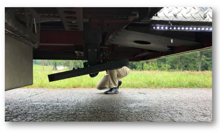
The pad is built into the bottom of the rear downrigger. Notice how the downrigger stows at an angle to improve angle of departure, but yet still hangs down. This could be an expensive repair if hit just right.
