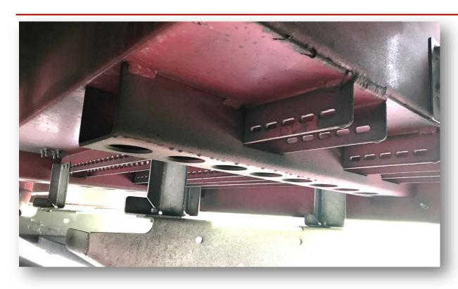
Notice the formed body compartment support members with lightening holes.
