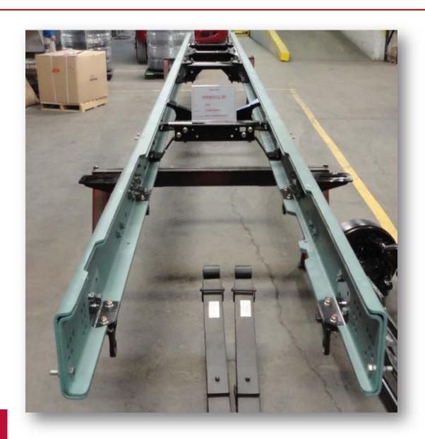
All Sutphen rear-mount aerial apparatus use Domex steel chassis frame rails with a true full-length 3/8" thick inner liner for strength.
