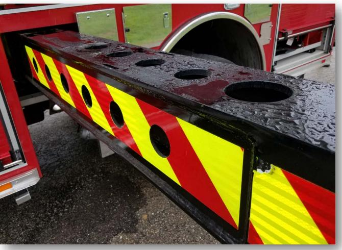
Notice the lightening holes in the top and sides of the outriggers.
