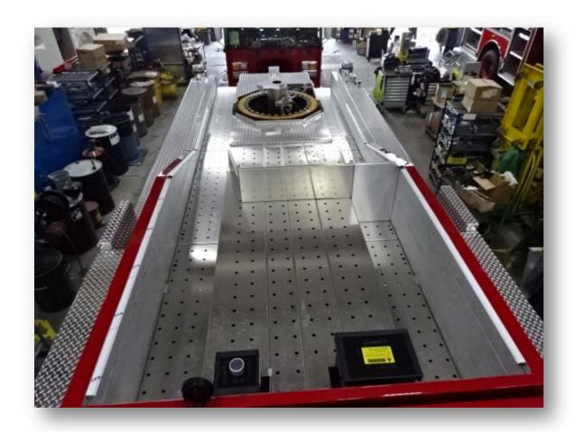
To fit 1000' of 5", the hose has to be loaded in front of the turntable area across the width of the truck (depending on which body is selected). It is not a straight rectangular bed. They are also using a plain perforated flat sheet of aluminum to keep weight down, unlike the slatted flooring they use in their other aerial products. This area of the main hose bed is not flat. It is stepped up over the water tank, making loading hose more challenging.
