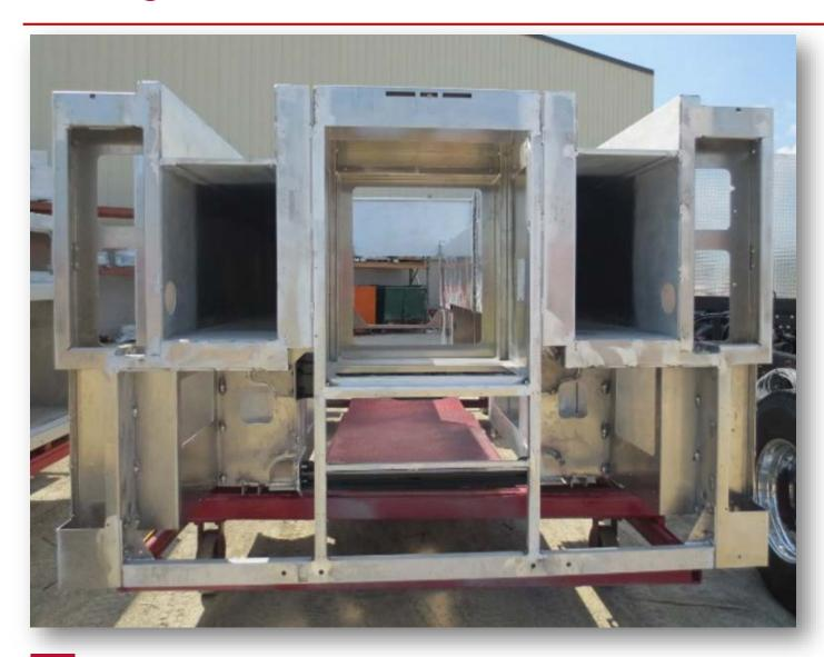
To reduce weight, they are using a self-supporting aluminum body (mostly just formed 1/8" sheet with some extrusions) that is attached to the torque box in only 3 places. There is no dedicated substructure to support the body.
