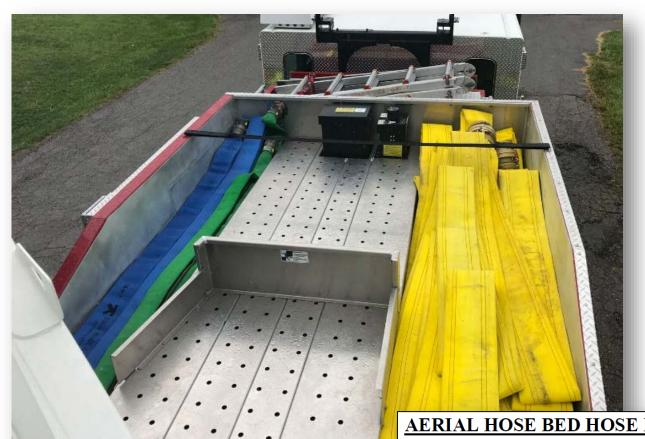
This image is of the Texas Chute Out style body which allows for all of the LDH to be on the officer's side. If using the quint body, one whole side plus part of the opposite side (including the middle section) are needed to achieve the advertised hose loads.
