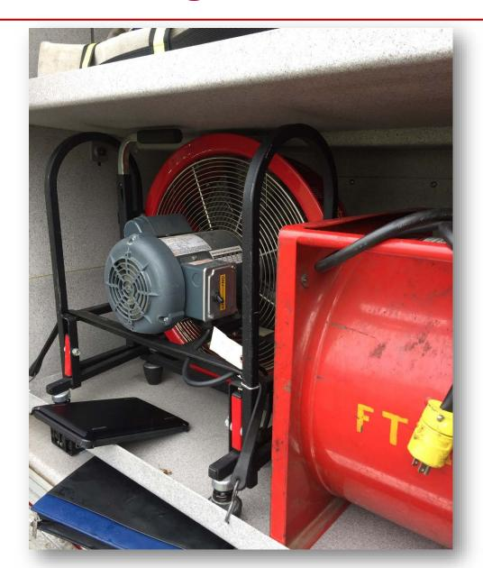
This is an older Tempest 16" fan. It barely fits in the compartment before it contacts the compartment notch.
