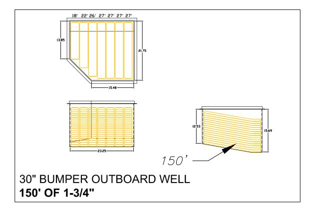
NOTE: CAPACITIES SHOWN DO NOT ACCOUNT FOR SWIVELS, NOZZLES, OR ADD'L CAPACITIES INSIDE RAISED LIDS. CAPACITIES SHOWN ARE ESTIMATIONS ONLY. CHARACTERISTICS OF EACH BRAND OF HOSE AND METHOD OF LOADING WILL DETERMINE TRUE CAPACITY.
