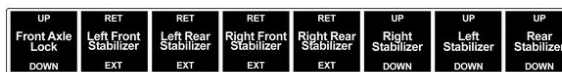
Sutphen Tag 406-A IC Label P/N 3001035-0001 Manual Override Outrigger Controls Label 50% Scale
