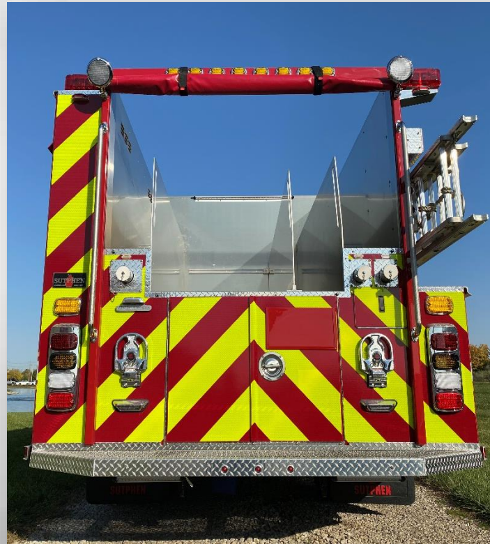
Modified hosebed with multiple rear discharges
