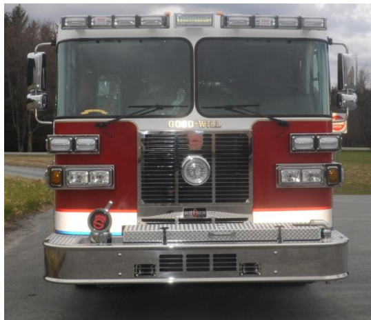
Goodwill HS5065 ISX Flat Roof A/C Condenser mounted in body Warning lights mounted to brow
