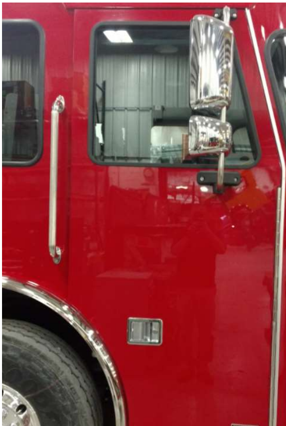
Exterior stainless handrails:
