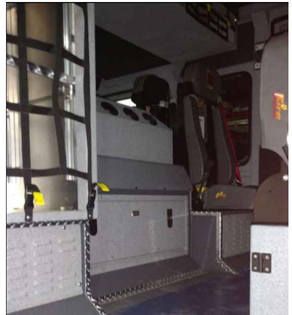
Small profile engine enclosure/tunnel (8" notch for additional leg room in crew cab):
