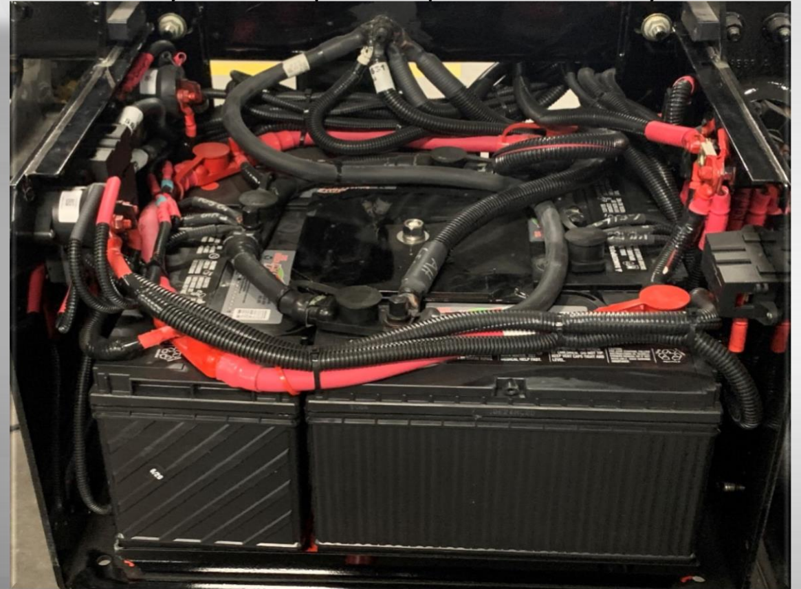
Battery box with point to point electrical system
