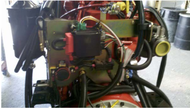
ECM, TCM, DCU RELAY/POWER DISTRIBUTION MODULE LOCATED ON THE ENGINE ACCESSORY PLATE
