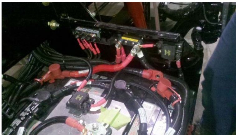
LOWERED CURRENT CIRCUIT BREAKERS AND REMOVED FROM BATTERY BOX
